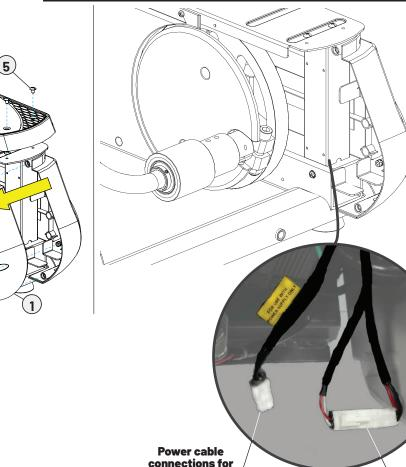
Power cable connections for consoles requiring optional power supply
